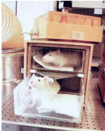
Figure 13: The experimental setup of Professor Salford showing TEM-cells (Salford, various publications)
